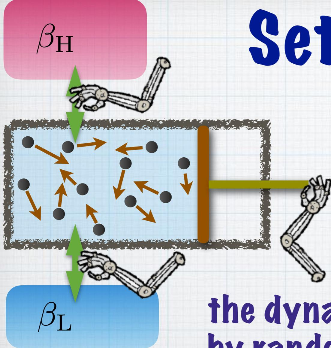
the engine is modeled as a classical system of  $N$  particles with arbitrary potential and interactions
